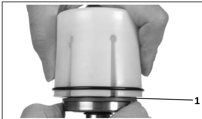
1. Seal installed in groove of piston
