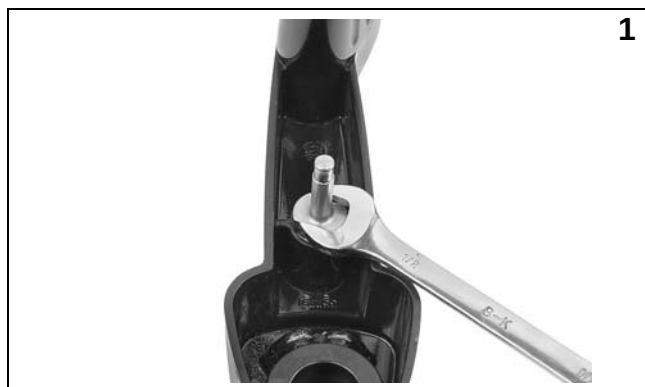
1. Detent ball, spring and guide
