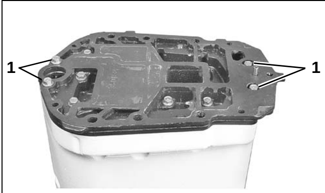
1. Adapter retaining screws
