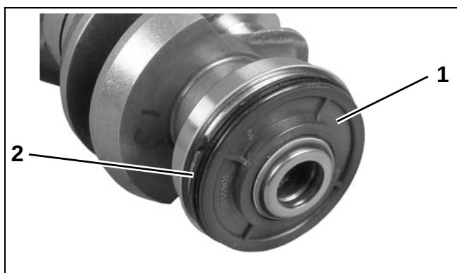
1. Lower seal housing 2. O-ring
