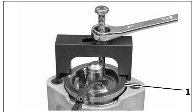
1. Fuel injector removed from fuel injector housing
