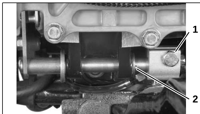
1. Shift rod lever screw 2. Cotter pin
