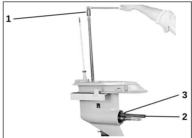
1. Holding socket 2. Pinion holder 3. Retainer
