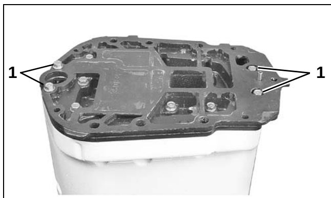
1. Adapter retaining screws
