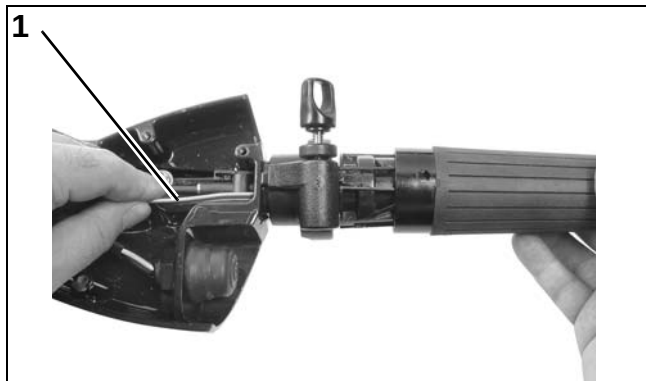
1. Trim switch wiring
