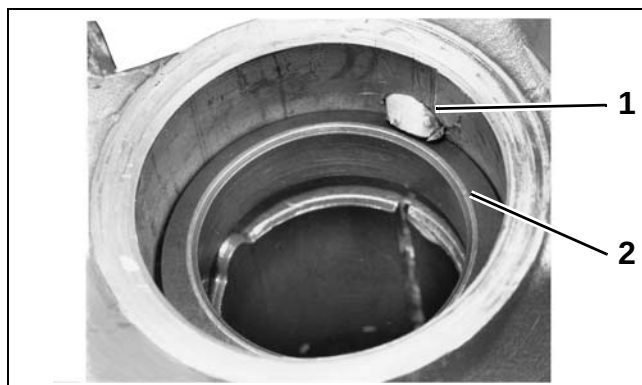
1. Steering friction pin 2. Steering friction thrust ring
